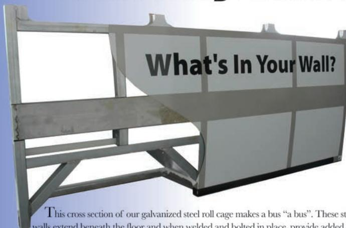
This cross section of our galvanized steel roll cage makes a bus "a bus". These steel side-walls extend beneath the floor and when welded and bolted in place, provide added strength and safety in the event of an accident. It may seem strange, but we spend considerable time thinking about safety, because although your passengers take it for granted, we can't. That's why we build it in from the ground up, then test it—specifically the FMVSS 214 side impact test.
